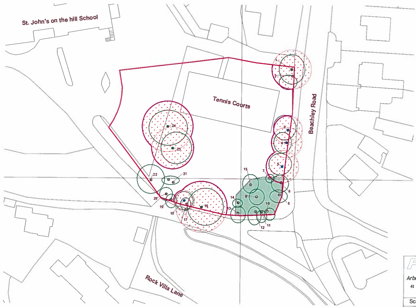
Plan 2: Plan to show the Root Protection Areas for retained trees at St John's Hill School, Castleford Hill, Tutts Hill, Chepstow, NP16 7LE. The locations for the positions of tree protective fencing is shown around the perimeters of all trees identified with Retention Category A or B.
